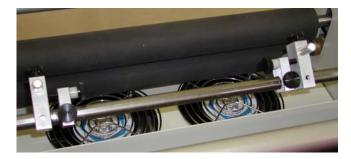
Included in the white box with your laminator are the slitter blades, do not install them unless you are using them, always remove them after use, they are a component as shown below and should be stored in a separate container (white shipping box) with a lid.
