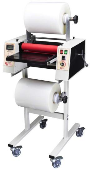
Using 2-3 people carefully the laminator on top of the stand, align the inside of the stand with the inside of the panel that sits on it, align the front of the stand with the front of the panel. Install the <sup>1</sup>/<sub>4</sub>-20 hex head screws with their respective washers through the holes in the top rail. DO NOT tighten these screws.
